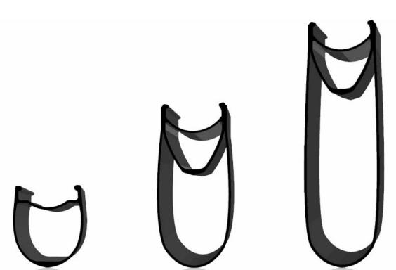
Wide rim shapes and brake tracks, improve aerodynamics, reduce the effects of side winds and improve rolling resistance.
