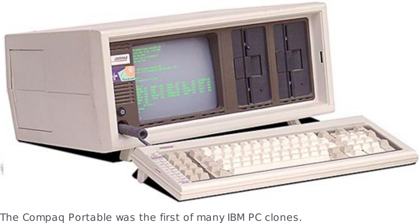
The Compaq Portable was the first of many IBM PC clones. oldcomputers.net
