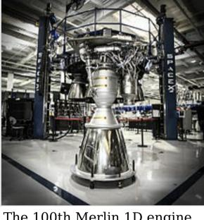
The 100th Merlin 1D engine, built at SpaceX's Hawthorne factory in 2014. The engine is already attached to its Octaweb load plate, for positioning in a Falcon 9 as one of eight outer engines.
