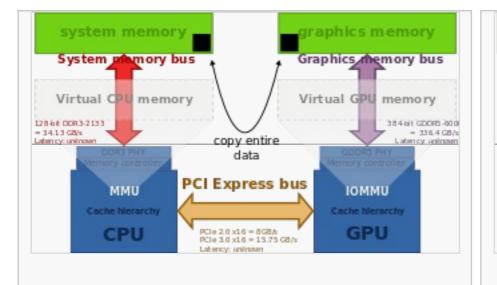
Classical desktop computer architecture with a distinct graphics card over PCI Express. CPU and GPU have their distinct physical memory, with different address spaces. The entire data needs to be copied over the PCIe bus. Note: the diagram shows bandwidths, but not the memory latency.
