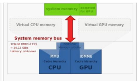
Integrated graphics-solutions (and <u>AMD APUs</u> with <u>TeraScale graphics</u>) suffer under *partitioned main memory*: a part of the system memory is allocated to the GPU exclusively. Zero-copy is not possible, data has to be copied (over the system memory bus) from one partition to the other.
