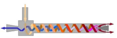
Separation of a compressed gas into a hot stream and a cold stream
