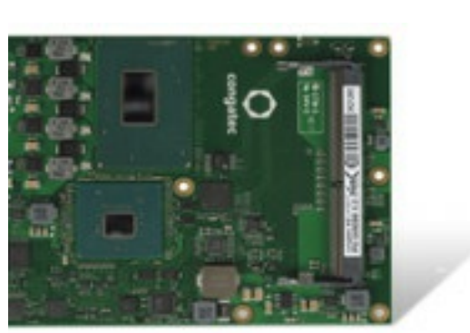
New congatec COM Express Computer-on-Module with 3 GHz Intel® Core™ i3 processor
