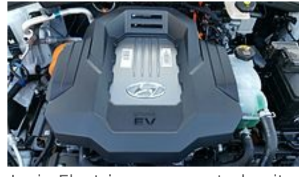
Ioniq Electric power control unit on top of the electric motor
