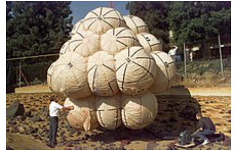
A test version of the Mars Pathfinder airbag system
