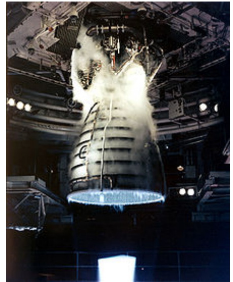
A remote camera captures a close-up view of an RS-25 during a test firing at the John C. Stennis Space Center in Hancock County, Mississippi .
