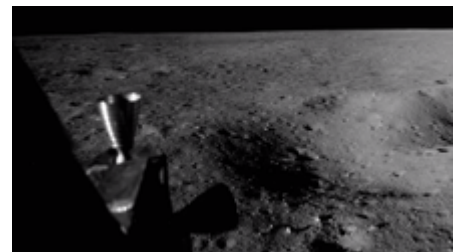
Bipropellant rocket engines of the Apollo Lunar Module reaction control system (RCS)
