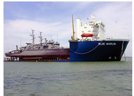
Blue Marlin transporting the U.S. Navy minesweepers USS Raven and USS Cardinal .
