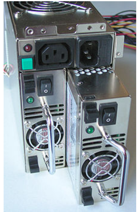
Redundant power supply contains two (or more) modules.
