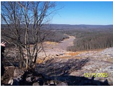
A broad swath of dense forest was washed away and scoured to bedrock by the escaping flow.
