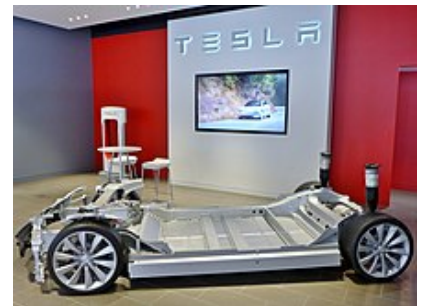
Tesla vehicle chassis used in Model S and X , with the battery visible
