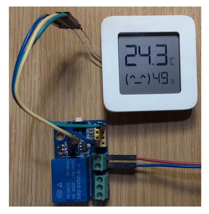
Trigger and reed switch status receiver on JDY-10 module (\$1).
