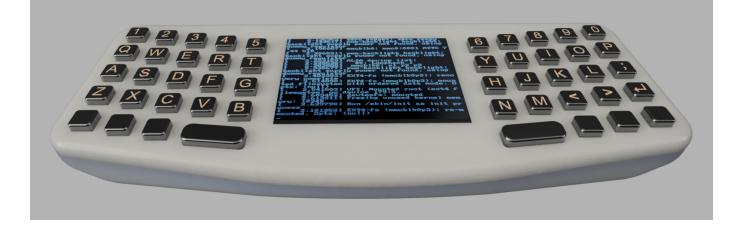
This is a 'Linux Swiss Army Knife', offering maximum utility while still being able to fit in your pocket. Is it fast? No. Can it run a GUI? Also no. But it can run scripts, ping a server, toggle a few GPIOs, and interact with a USB device. This is a minimum viable computer that can:
