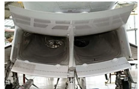
S-duct-like air intake conceals engine fans, a major source of radar wave reflection
