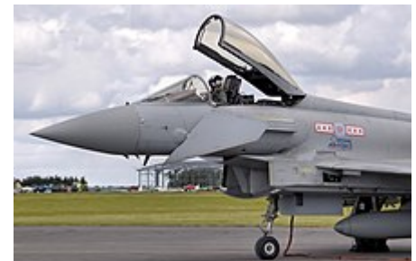
Close-up view of RAF Typhoon F2 ZJ910, showing the deflected canard control surface immediately below the pilot
