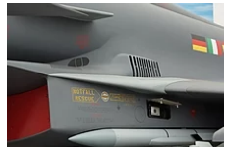
AMK Leading Edge Root Extension
