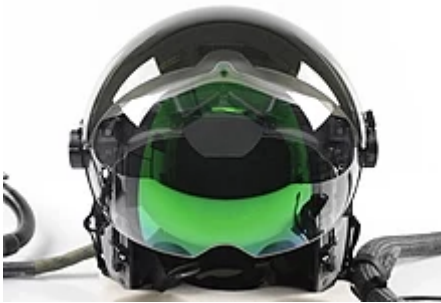
Helmet Mounted Symbology System (HMSS)
