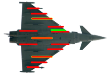
The Eurofighter Typhoon has 13 hardpoints for carrying armament
