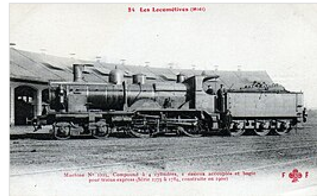
Locomotive 220 1775 compound à 4 cylindres, 1900.
