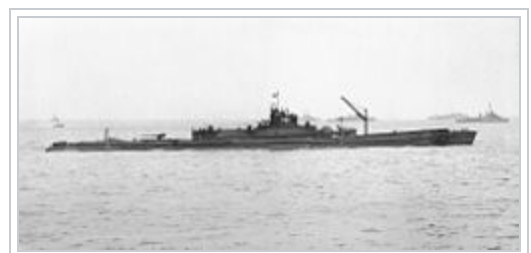
An I-400 class submarine, with its long plane hangar and forward catapult
