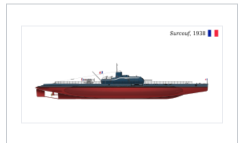
1938 configuration: radio mast removed and different conning tower
