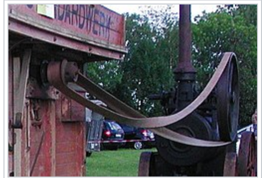
The drive belt: used to transfer power from the engine's flywheel. Here shown driving a threshing machine .
