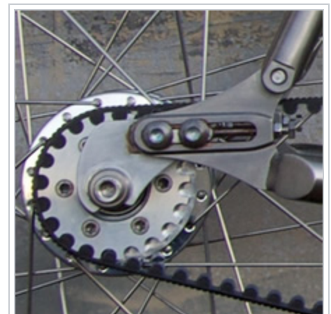
Belt-drive cog on a belt-driven bicycle
