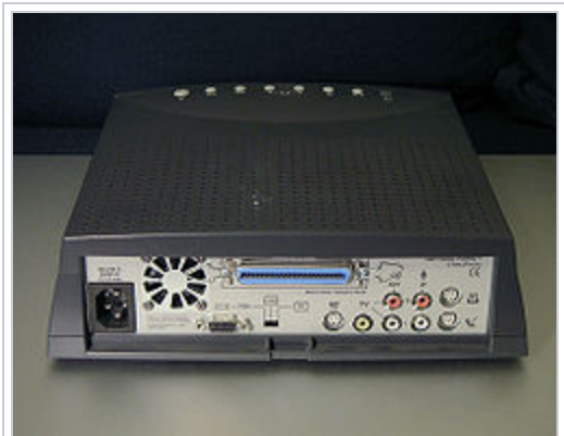
The rear of the Katz Media KMP 2000 has a unique external SCSI interface.
