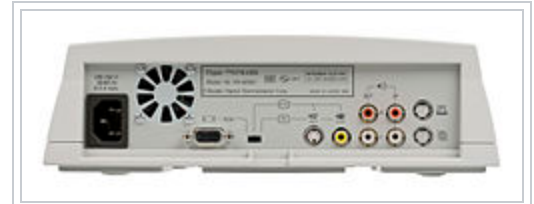
The rear panel of the Pippin has multiple A/V outs and printer and modem ports.
