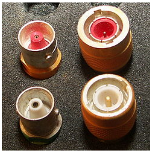
50 \Omega (white/bottom row) and 75 \Omega C connectors (red/top row)
