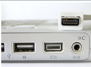
Male Mini-VGA plug on top of an Apple laptop, female port is second from right.
