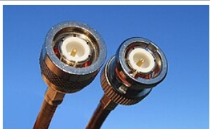
TNC connector (left), compared with BNC (right)
