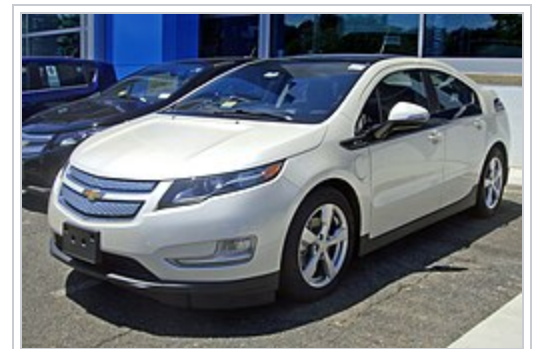
The Chevrolet Volt is a series plug-in hybrid referred by General Motors as "an electric car with extended range."
