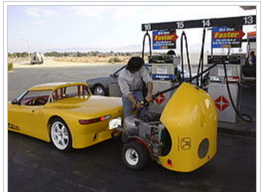
A prototype AC Propulsion tzero electric car with an external range-extender or genset trailer, 1999
