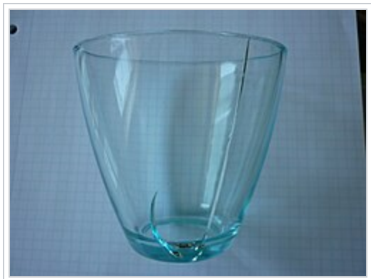
Drinking glass with fracture due to uneven thermal expansion after pouring of hot liquid into the otherwise cool glass
